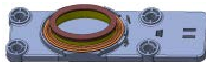
Fig. 17. Design Model of Ellipse Type Single Core Exciter
